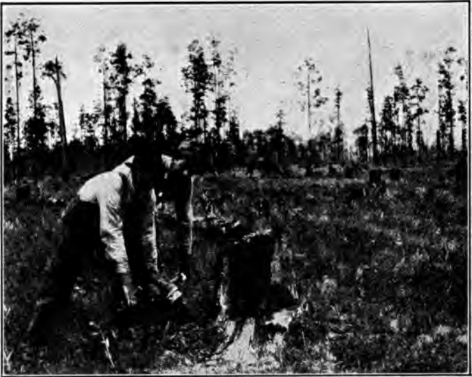
Fig. 24. Boring a Long-Leaf Pine Stump with an Electric Drill
